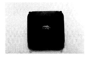
process, the circuit board is embedded in a plastic plate (Figure 3 above) that will later be trimmed to fit the custom shell of the hearing aid.
